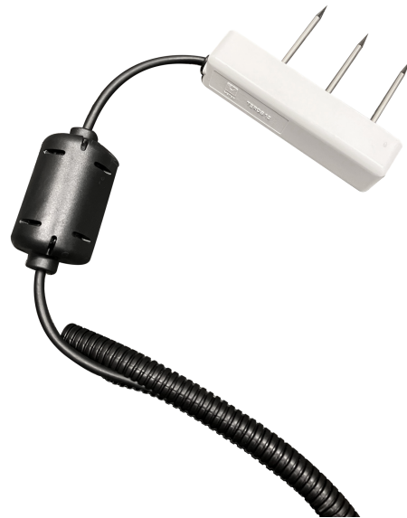
Figure 20. Cable protector on soil probe cable
