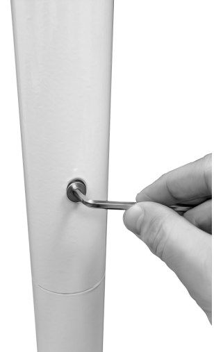
Figure 13. Securing pole fasteners
