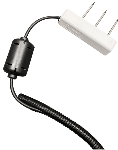
Figure 20. Cable protector on soil probe cable
